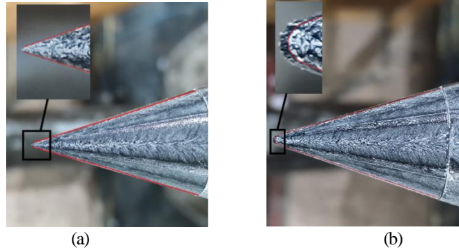
Fig. 2 Two patterns of separation over the slender bodies with different nose shapes. (a) open-type separation at a pointed-nosed slender body with B=0 ; (b) close-type separation at a blunt-nosed slender body with B=3 .
